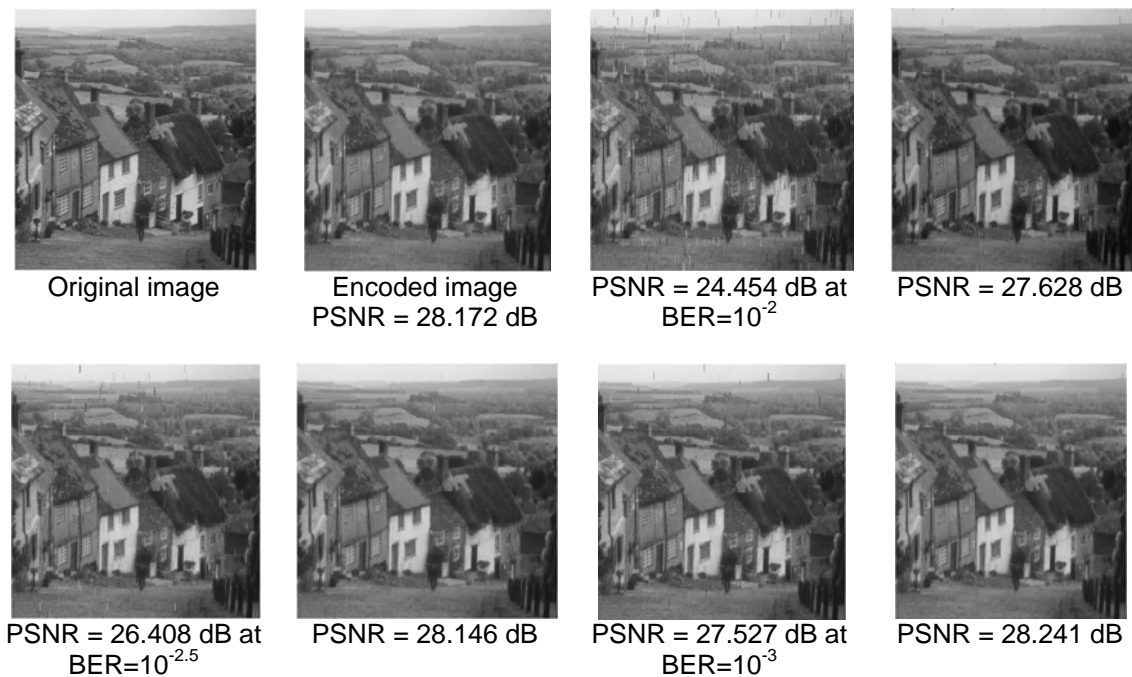
Figure 8. Restored Goldhill image at different BER using median filter (Left: Degraded. Right: Restored)
