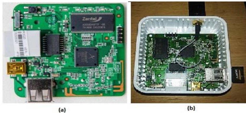
Figure 1. MR3020 Board a) Original Board b) MR3020 Modified
