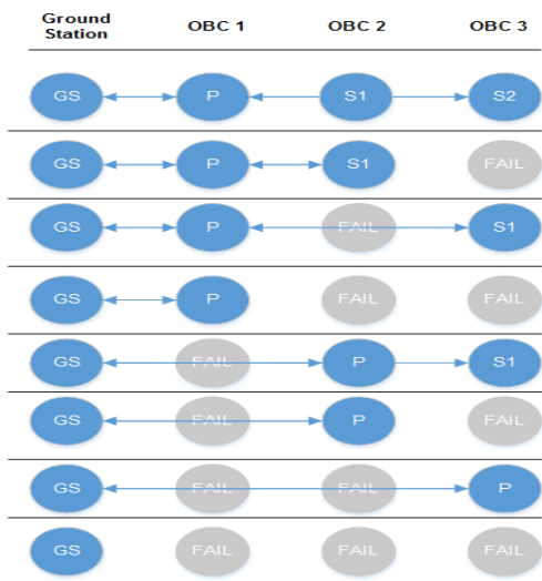
Figure 9 Redundancy Scenario: Disconnected with GS
