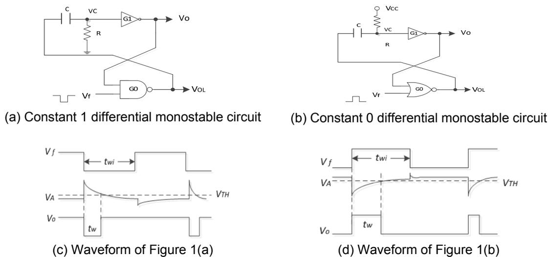
Figure 1. Differential monostable circuits and their waveforms
