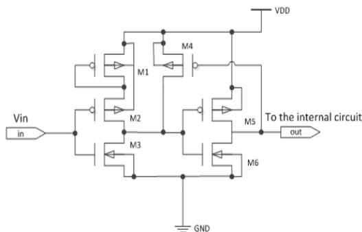
Figure 3. Level-switching circuit
