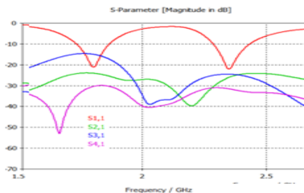
Figure 4. The effect mutual coupling Port 1 of Port 2
