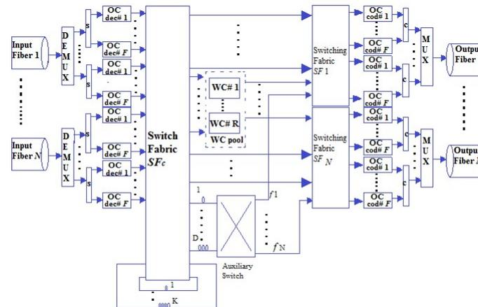
Figure 1. Architecture of OCDM/WDM with shared FDL.
