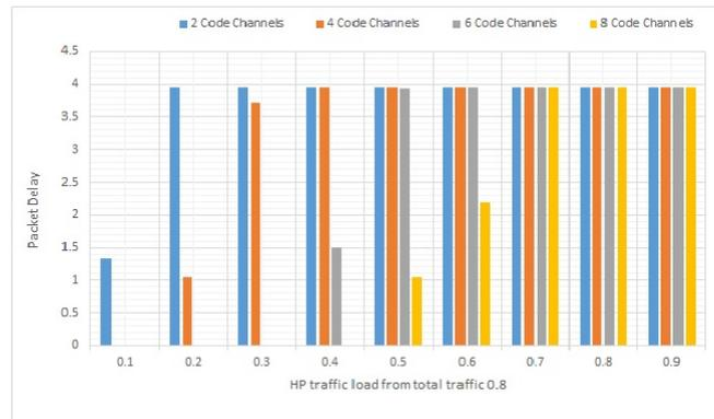
Figure 7. Packet Delay of HP hybrid OCDM/WDM system versus a variety of HP traffic from total traffic 0.8, for different numbers of channels reserved to HP, shared input privet output mechanism.
