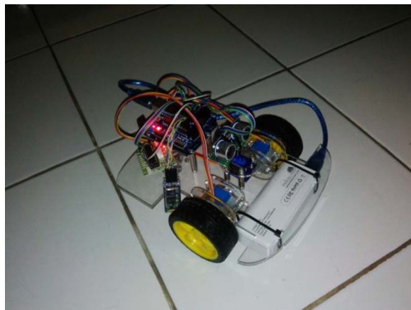
Figure 2. Sonar sensor mounted on servo
