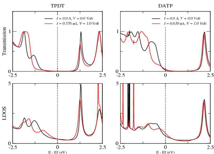
Figure 2. Local density of states and Transmission of TPDT and DATP molecules in equilibrium and under applied bias
