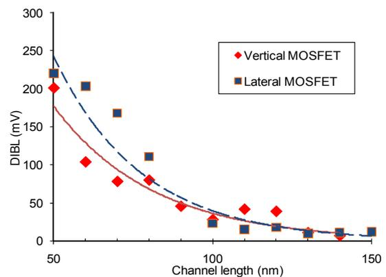
Fig. 3 Trend of DIBL for lateral and vertical MOSFET
