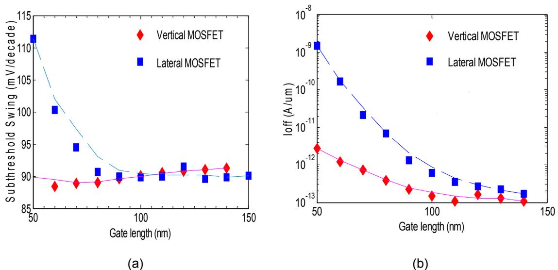
Fig. 4 (a) Subthreshold swing (SS) of vertical and lateral MOSFET for channel length= 50-150 nm, and (b) the leakage current ( $I_{off}$ ) of both structures (taken at  $V_g=0V$ )
