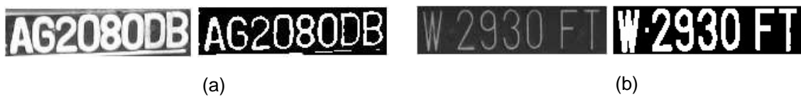
Figure 10. The dilation morphological process, (a). large character and its erosion result, (b) small character and its dilation result
