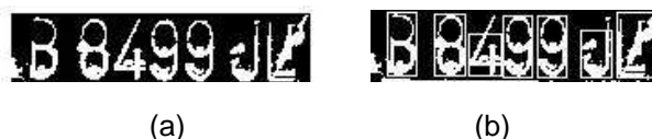
Figure 15. The real-time experiment, (a) license plate image with noise, (b) segmentation result
