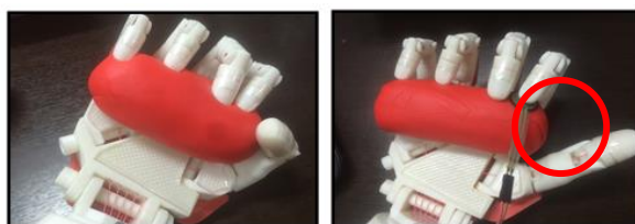
(a) (b) Figure 14. Grasp Play-Doh with and without feedback
