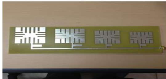
Figure 5. Fabrication of microstrip antenna design
