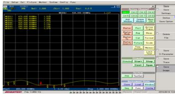
Figure 7. Measurement of VSWR
