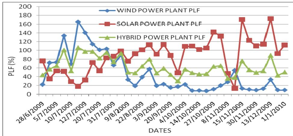
Figure 2. Comparison of actual PLF of wind, solar and hybrid power plant
