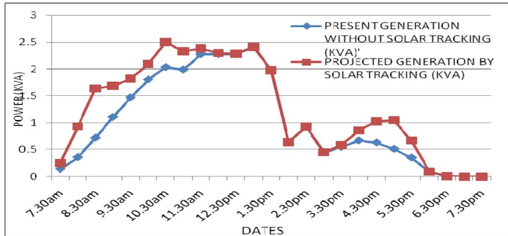
Figure 4. Comparison of actual and projected generation by SPV cells with solar tracking
