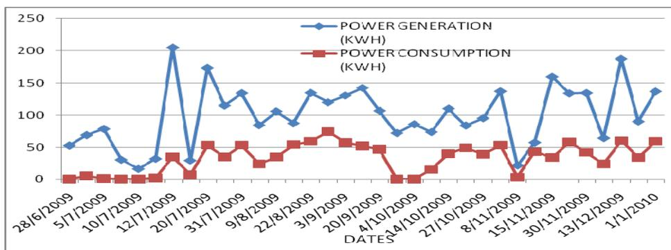
Figure 1. Total generation by the hybrid power plant and consumption of this power
