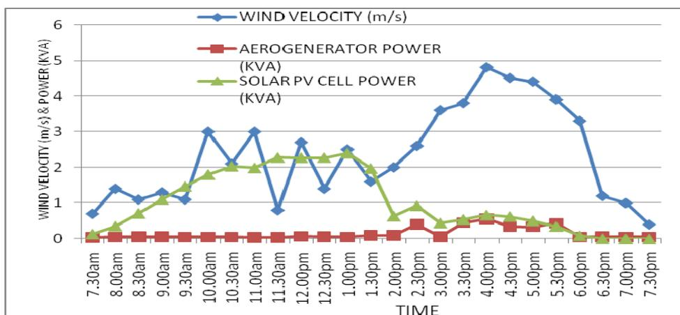
Figure 3. Wind velocity, solar and wind power generation in a day
