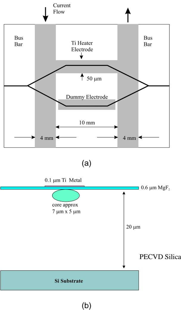
Figure 1. (a) Layout of thermo-optic Mach-Zehnder interferometric switches, (b) Cross section of a straight guide of a Mach-Zehnder interferometer with an  $\text{MgF}_2$  cladding layer and an additional Ti heater
