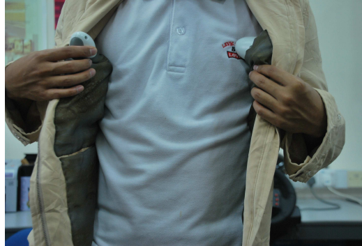
Figure 4. Wearable haptic with four haptic devices attached to the jacket
