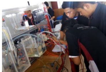
Figure 9. Wiring process using process control laboratory kit
