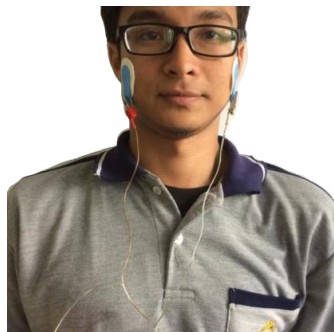
Figure 7. Electrode positions of EMG sensor
