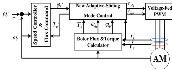
Figure 2. The Overall Simulated Block Diagram of the Proposed New Adaptive Sliding Mode Control
