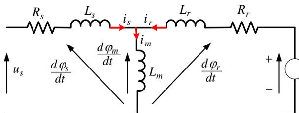
Figure 1. Equivalent Circuit of an Asynchronous Motor
