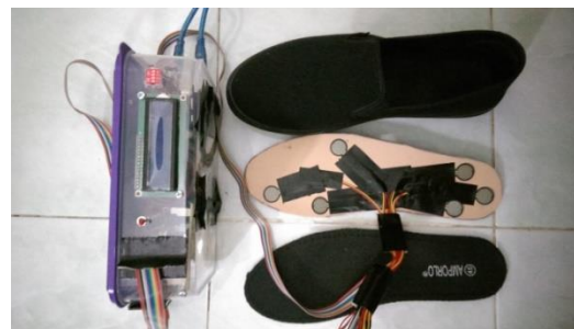
Figure 4. Final Product of DAQ Hardware
