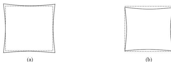
Figure 1. (a) Showing effect of negative and (b) positive pincushion distortion on images. The dashed line represents the actual image without any distortion.
