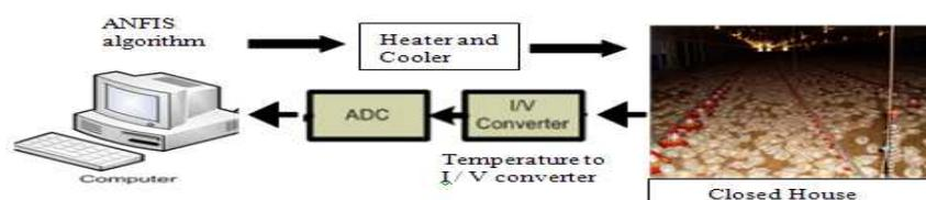
Figure 1. Closed house system for broilers (Cikabayan Unit University of farm IPB, 2009)
