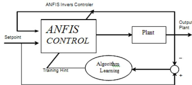
Figure 3. Block diagram control of ANFIS
