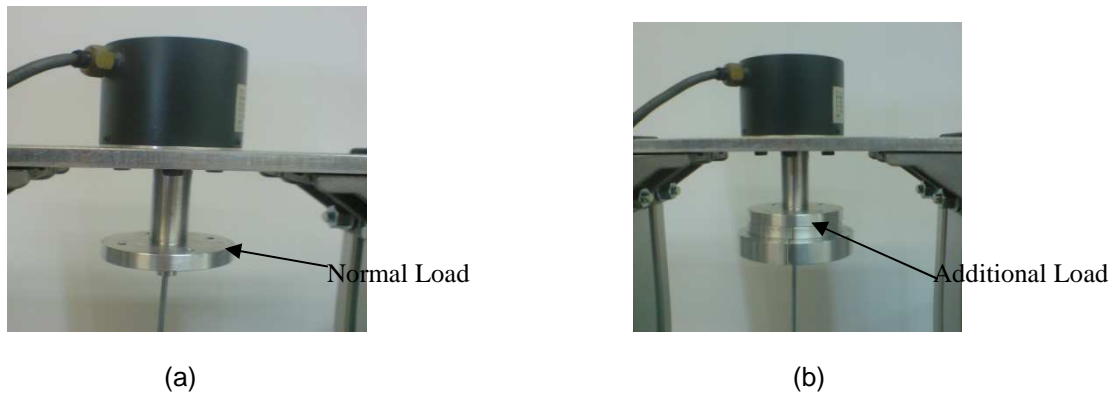
Figure 8. Nominal and increased object inertia: (a) Normal object, (b) Increased inertia object
