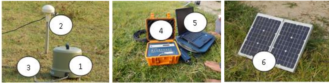
Figure 2. Primary data acquisition tools: (1) triaxial geophone; (2) GPS; (3) sensor cable; (4) seismic data digitizer and recorder; (5) laptop; (6) solar cell panel
