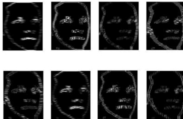
Figure 3. The upper row images are the results using Gabor filters with the window size of (2, 1), and the orientation of 2\pi/12 , 5\pi/12 , 8\pi/12 and 11\pi/12 respectively. The lower row images are the results using Gabor filters with the window size of (4, 2), and the orientation of 2\pi/12 , 5\pi/12 , 8\pi/12 , 11\pi/12 respectively
