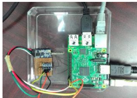
Figure 5. Hardware of the Access Point
