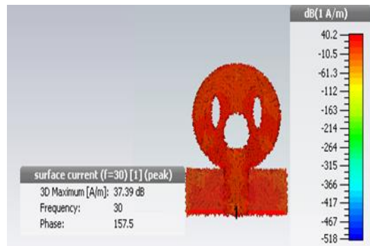
(f) Current surface distribution at f=30 GHz
