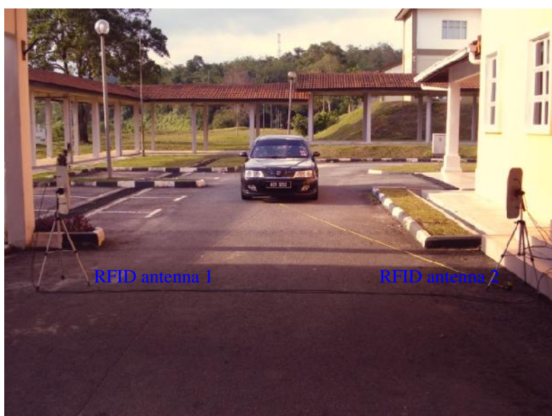
Figure 9. Field testing of proposed e-plate antenna installed on vehicle.
