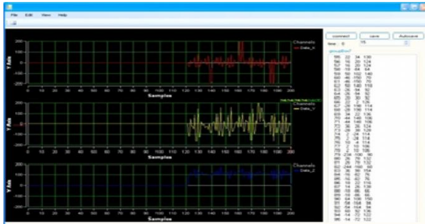
Figure 8. Vibration data plotted in the time domain signal
