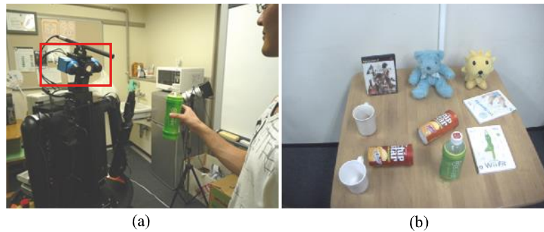
Figure 3. (a) Object learning scenario: a user is showing the target object to the robot [12], whereas the red rectangle depicts the 3D visual sensor proposed in [11], and (b) examples of objects used in the experiment.
