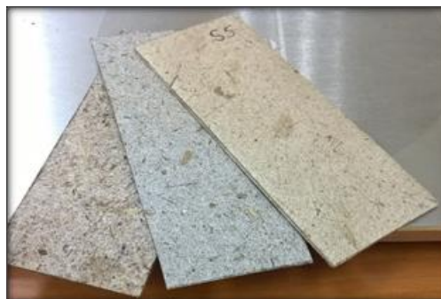
Figure 1. Proposed paper substrate materials for microstrip reflectarray antenna
