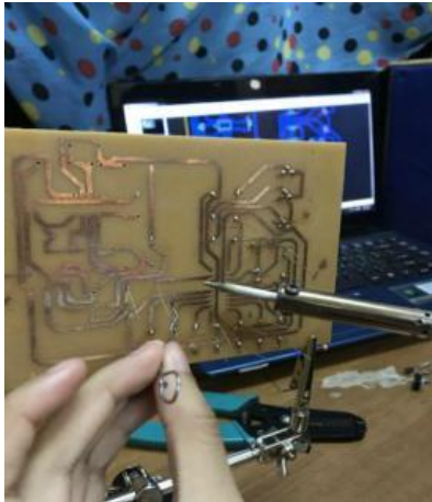
Figure 10. Construct and solder component
