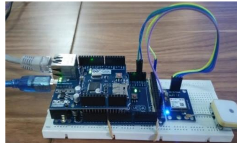
Figure 4. GPS NTP server based on arduino mega 2560
